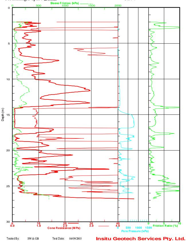
Tested By: SW & GB Test Date: 04/09/2003 IGS No: 1367 Job No: 0309-01 Tested in accordance with AS 1289.6.5.1 -1999. Page No: 1 of 1
