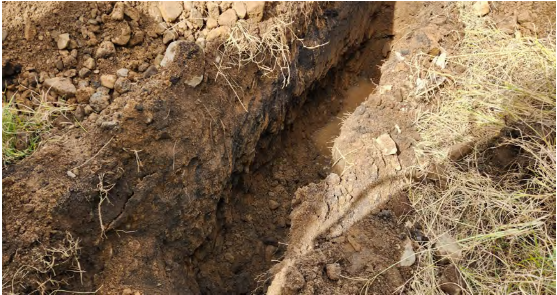
TPL-05 - 1: Test pit excavation - sidewall collapse occurring at depth of water inflow
