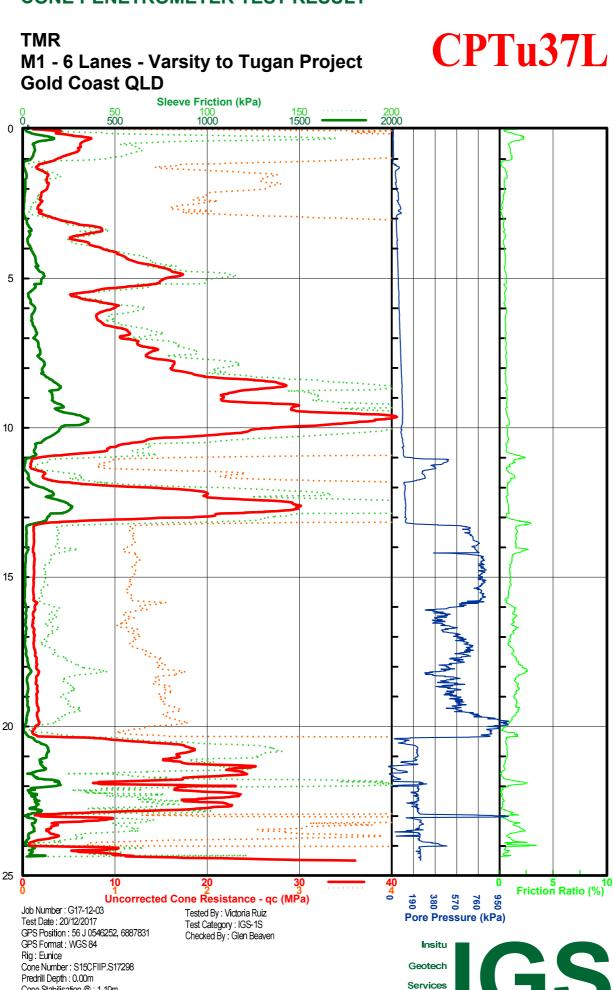
Cone Stabilisation @: 1.19m Cone Dissipation @: 14.18m Terminated Due To: Equipment at Risk
